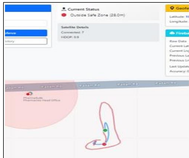
Fig 4 System Alert Displayed when the Tracked Device Breaches a Geofence Boundary
