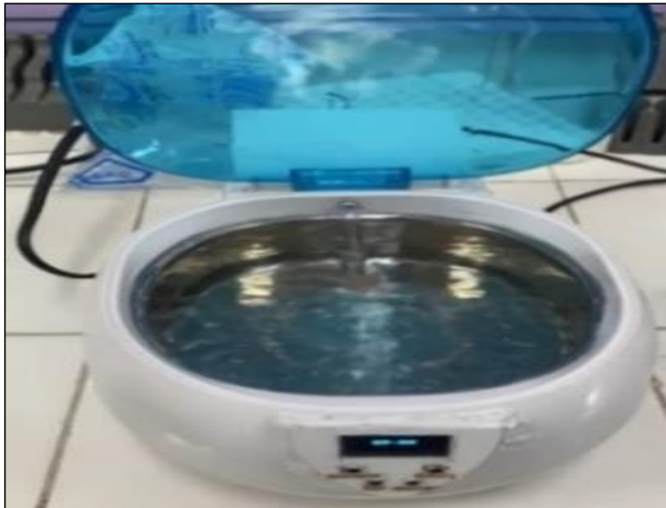
Fig 2 Dental Prosthesis Cleaner with Ultrasonic Technology in the on State
