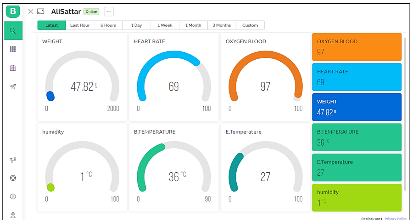
Fig 4 Real-Time Infant Incubator Monitoring Through the Blynk IoT GUI on a Computer.
