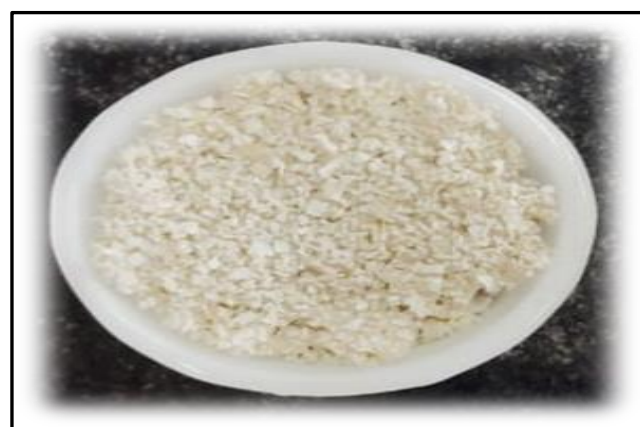
Fig 3 Chicken Egg Shell Powder, 5% and 7% WT.
