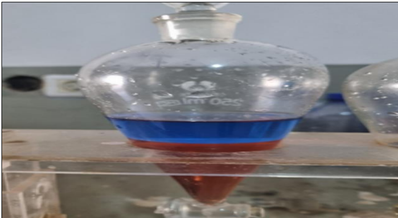
Fig 2 Presentation of Two Phases after Agitation (Extraction)
