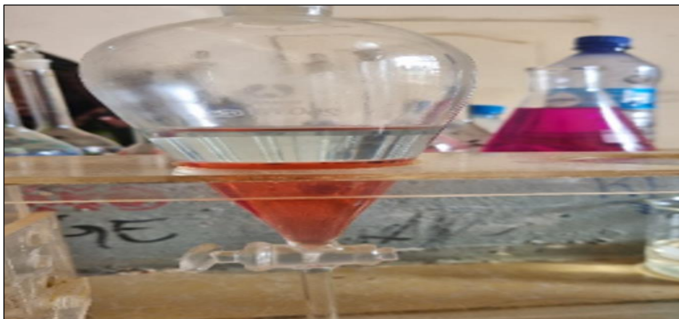
Fig 1 Presentation of Two Phases (Aqueous and Organic) in A Separating Funnel
